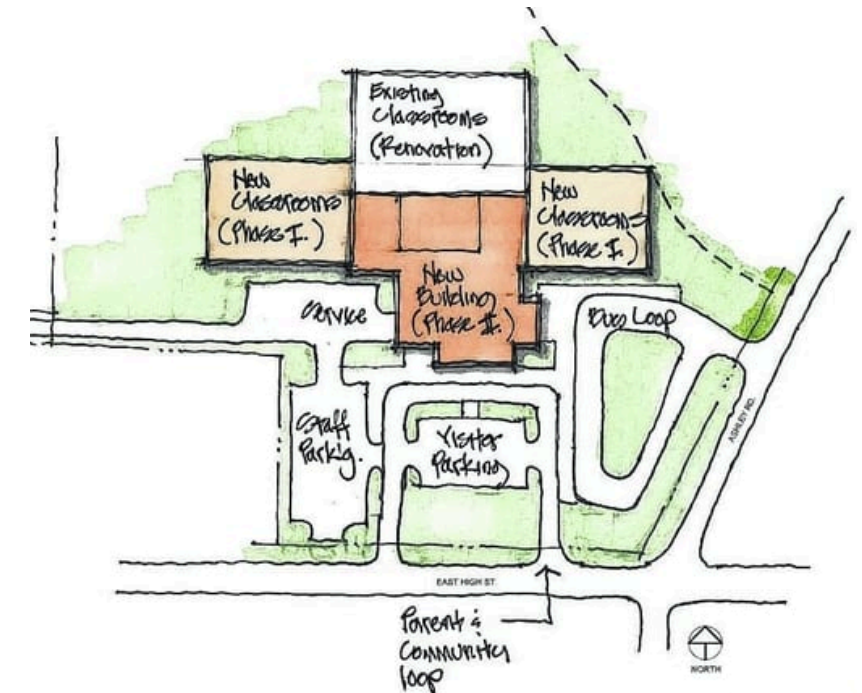
Example of a site plan that distinguishes various modes of vehicular traffic.
